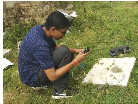
Figure 9. Temperature recording using digital indicator
